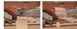
Fig. 2: The experimental setup includes a US transducer and a (Lego-built) safety device.
